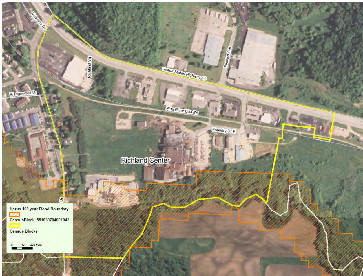
Figure 3a: Flood Damage Exposure in Richland
